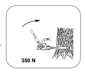
Do not strike the wedge into cut by force. Do not act on the wedge by external dynamic strokes.
