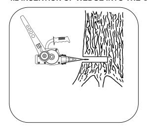
**CORRECTLY** – into the cut are inserted only the ends of elastic blades
