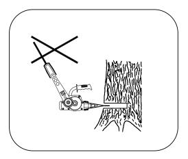
Do not use the wedge for tree felling of larger volumes, where the gravity centre is offset in direction of the main cut.
