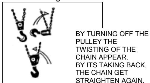
Obr. 2 Kinking of a chain
